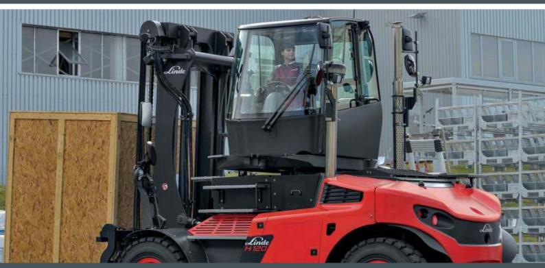
With the help of the rotating cab, the driver always has an optimum circumferential view. Compared to the standard model, the cab height is increased by 600 millimetres, and the cab can be rotated in infinitely variable stages using the joystick or the position switches by up to 180 degrees to the left or 65 degrees to the right.
